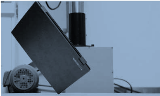
26 DIFFERENT WAYS TO DROP A NOTEBOOK: One MIL-STD 810G test requires devices to be dropped from 76 cm (the height of an average desk). We repeat the test from 26 different angles, looking for weaknesses and eliminating them. Tests are performed by an independent, third-party certification organization - TÜV Rheinland Japan.
